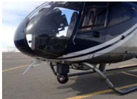
Helicopter with forward-looking infrared (FLIR) technology
