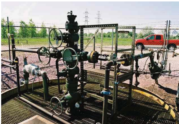
A Christmas tree at an oil well in Bay City, Michigan (Photo by Flow Research)
