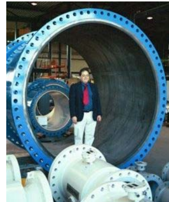
Dr. Yoder inside an 86 inch magmeter
